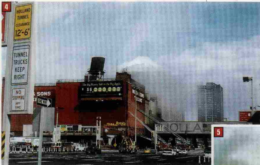
(4) Smoke is showing from stairwells at each corner of the building. Note the leaning water tower on top of the building. (5) Large cracks in the west wall show the heavy fire inside and helped lead to the IC's decision to withdraw personnel from the building.
